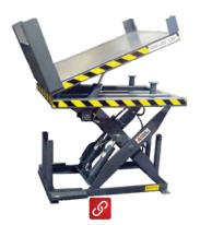
SSLT Lift / Tilt Series 0-45 degree tilt angle 2,000 to 10,000 lbs. capacities 24" x 48" to 60" x 108" platform sizes
