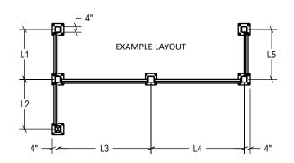
CENTER TO CENTER OF POST (L) = GUARDRAIL LENGTH + 4" OUTSIDE DIMENSION OF POST BASE = 4"
