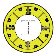
**STEP 3:** LAG THE COLUMN GUARD SECTIONS TO THE FLOOR USING PROVIDED ANCHORS AND SPECIFICATIONS
