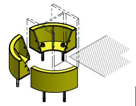
COLUMN GUARDS CAN BE MOUNTED SEPARATELY TO FIT AROUND LARGER ITEMS OR OMITTED TO AVOID OBSTACLES
