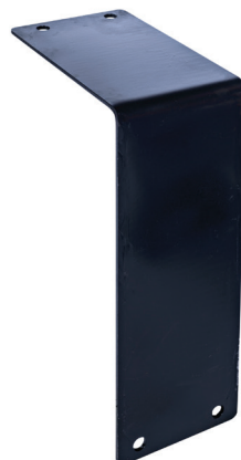
MOUNTING PLATE Used when the concrete at the bumper mounting location is damaged and preventing secure installation of dock bumper. The bumper mounting plate can be made wider and higher to allow fastening into more solid concrete. They can ship with the dock bumpers welded to them for easier one-step installation.
