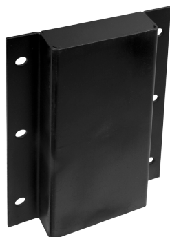
EXTENSION BRACKET Used when the dock bumper projection must be increased and it cannot be accomplished by choosing the bumper size of appropriate projection. They can also be used to extend an existing bumper to the proper projection. Extension brackets can ship with the dock bumpers welded to them for easier one-step installation.*
