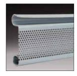
Secur-Vent® – Slat consists of 1/16"diameter hole offering 20-25% open area over length of each slat. Available in galvanized steel, stainless steel and aluminum.
