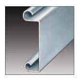
No. 17 – 2" Flat-faced slat up to 20-gauge steel, 20-gauge stainless steel, or 16 B&S gauge aluminum (mill, clear, or bronze anodized). Depth: 1/2", 1-7/8" on centers.
