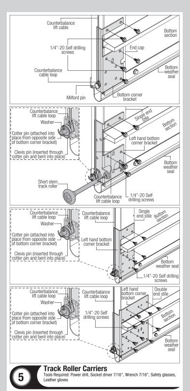
NOTE: If you don't have track roller carriers, then skip this step. Refer to Package Contents / Parts Breakdown, to determine if a track roller carrier was supplied with your door.
