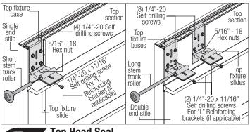
**Top Head Seal**Tools Required: Power drill, Phillips screwdriver, Saw horses, Tape measure, Safety glasses, Leather gloves
