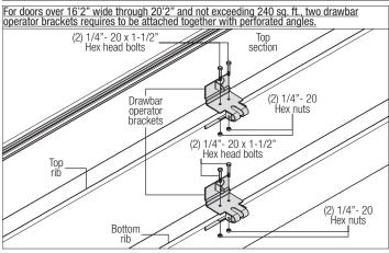
DRAWBAR OPERATOR BRACKET (RECTANGULAR): Locate the center of the top section
