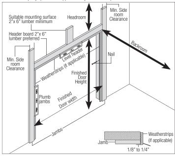
**HEADROOM REQUIREMENT:** Headroom is defined as the space needed above the top of the door for tracks, springs, etc. to allow the door to open properly. If the door is to be motor operated, 2-1/2" (64 mm) of additional headroom is required.
