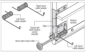
**Broken Cable Safety Device**
